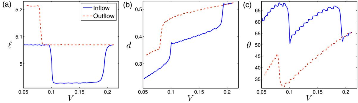
Figure 4: Numerical computations of a the different quantities characterizing the droplet dynamics as the volume is increased and decreased: displacement  $\ell$  (a), droplet base  $d$  (b), and one of the contact angles  $\theta$  (c). The wavelength of the chemical heterogeneity is  $\lambda = 20$ .
