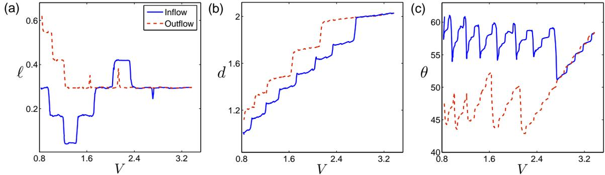
Figure 5: Numerical computations of a the different quantities characterizing the droplet dynamics as the volume is increased and decreased: displacement  $\ell$  (a), droplet base  $d$  (b), and one of the contact angles  $\theta$  (c). The wavelength of the chemical heterogeneity is  $\lambda = 100$ .
