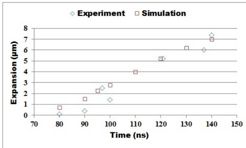
Figure 1. Comparison of diffraction imaging experimental vs FEM numerical results of wire's expansion
