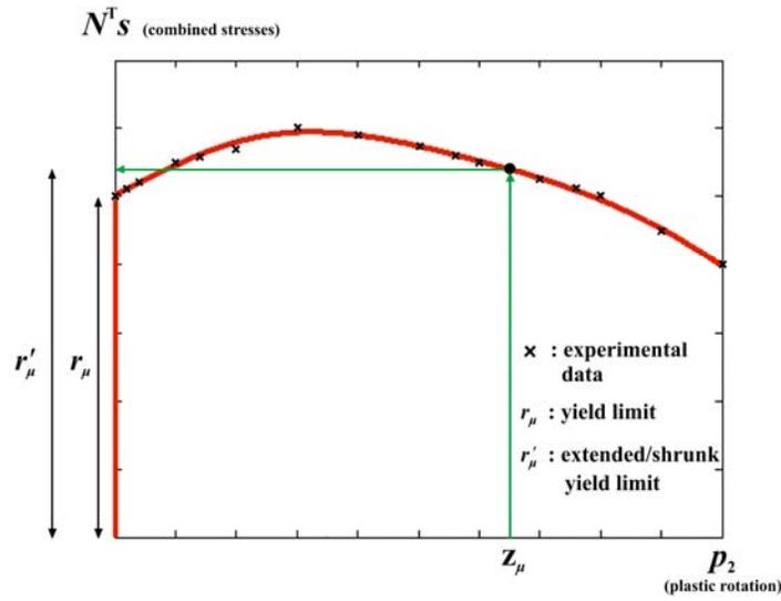
Figure 3: Nonlinear hardening/softening behavior using curve fitting tool.
