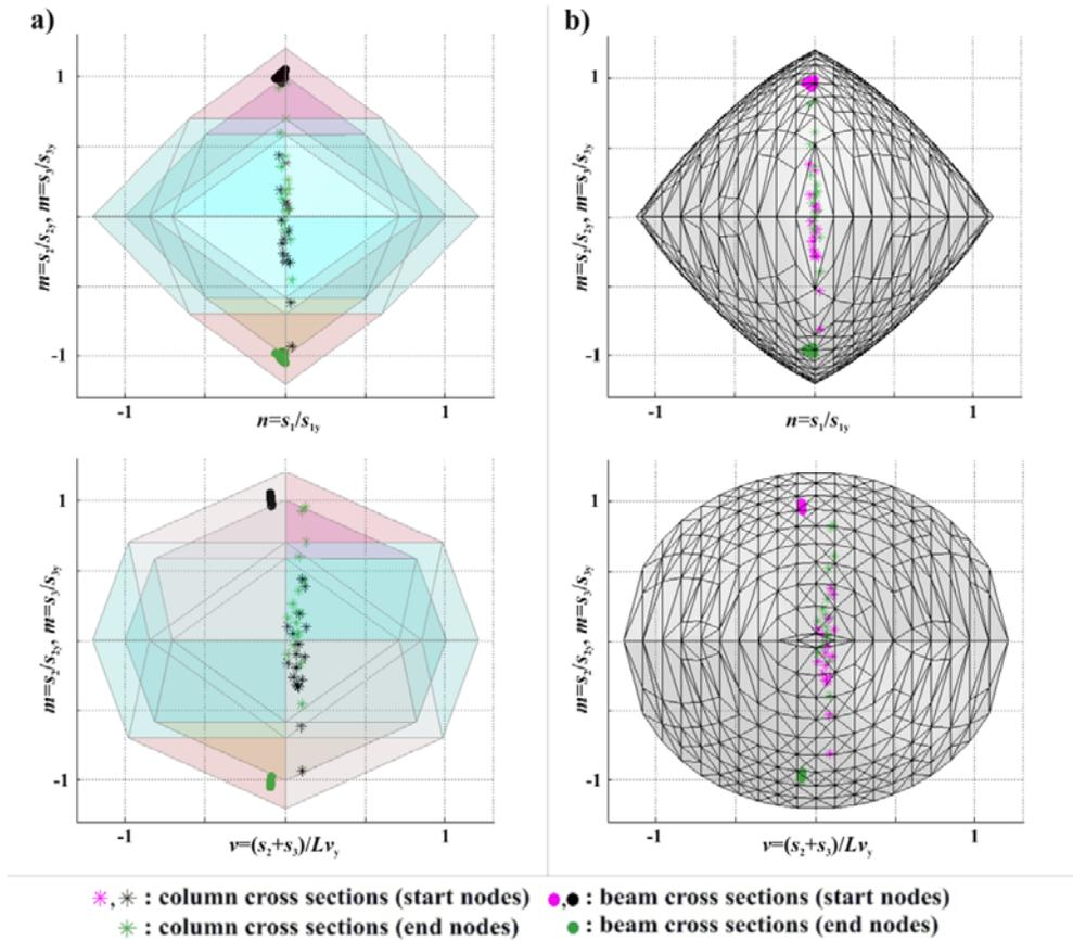
Figure 7: NQM interaction diagrams for a) case (b<sub>1</sub>) and b) case (b<sub>3</sub>).
