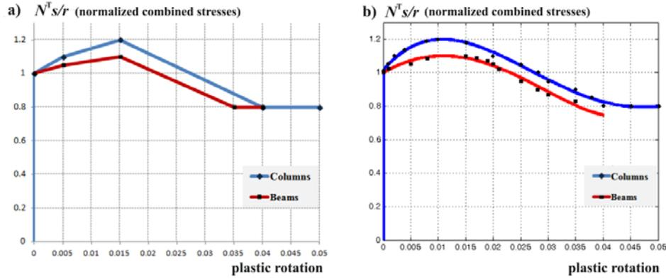
Figure 5: a) Multi-linear and b) nonlinear hardening/softening structural behavior.
