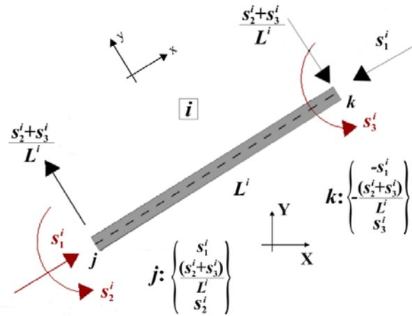
Figure 1. Frame element  $i$  with equilibrated stress resultants-end actions.
