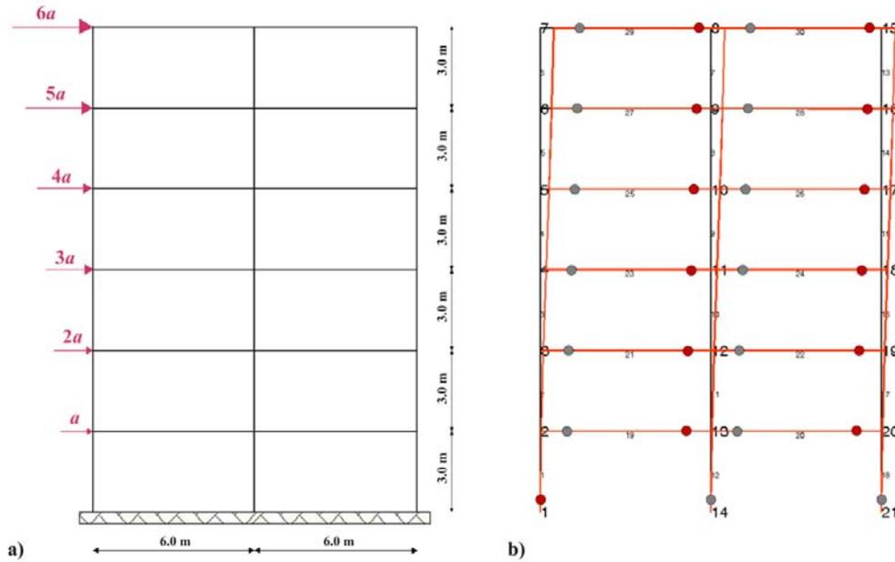
Figure 4: a) Three-storey, two-bay steel frame and b) plastic hinge formation for all analysis cases.
