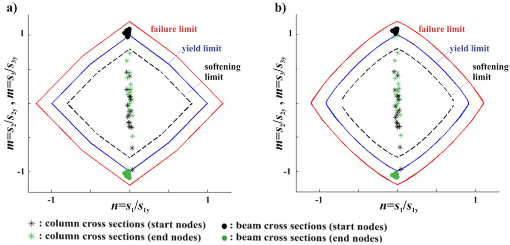
Figure 6: NM interaction diagrams for a) case (a<sub>1</sub>) and b) case (a<sub>3</sub>).
