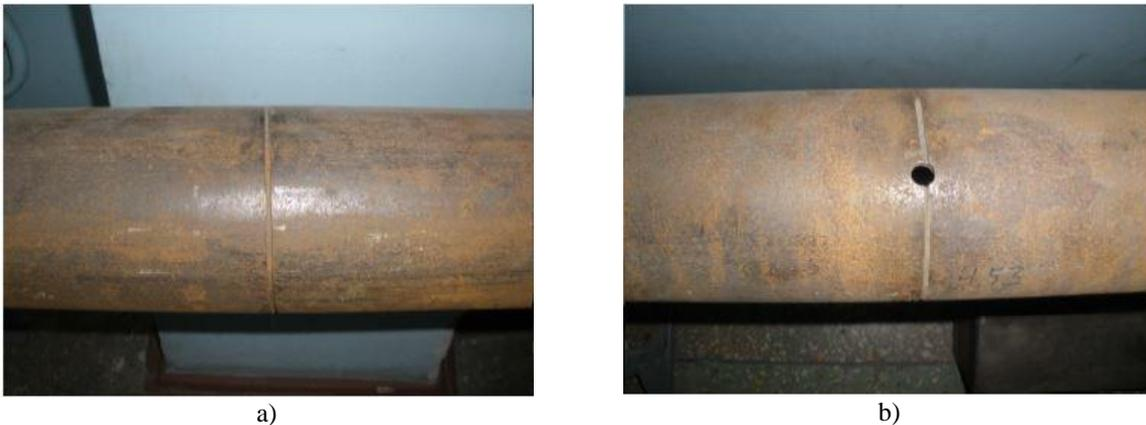
Figure 1. Two types of defects on a sample pipe: notch (a) and notch with a hole (b)
