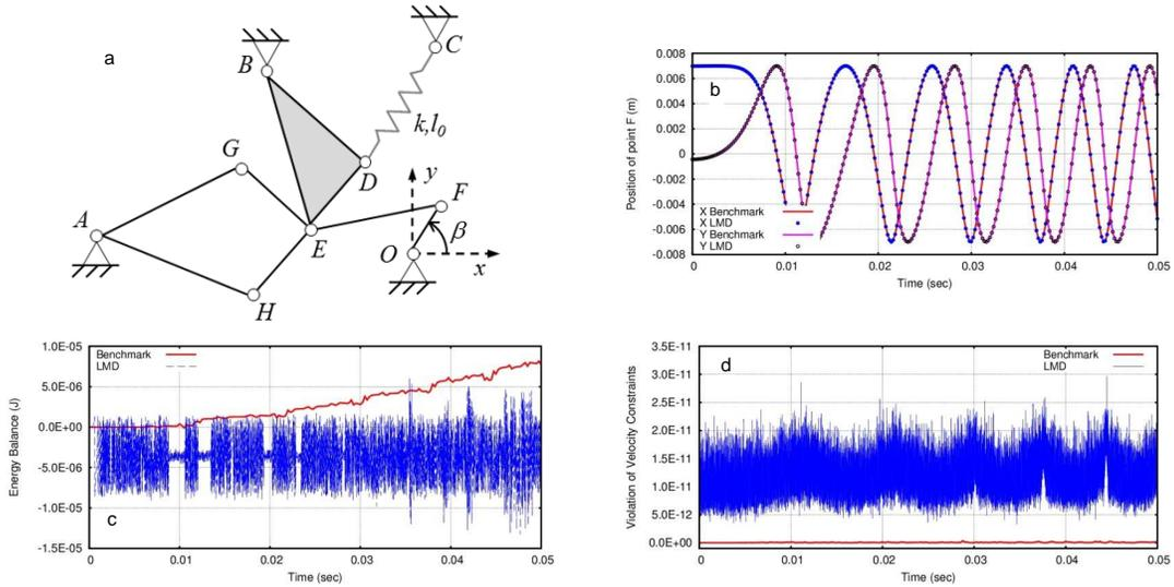
**Fig. 4.** (a) Mechanical model of Andrews' squeezer mechanism, (b)  $x$  and  $y$  coordinates of point F, (c) mechanical energy balance, (d) violation of velocity constraints.
