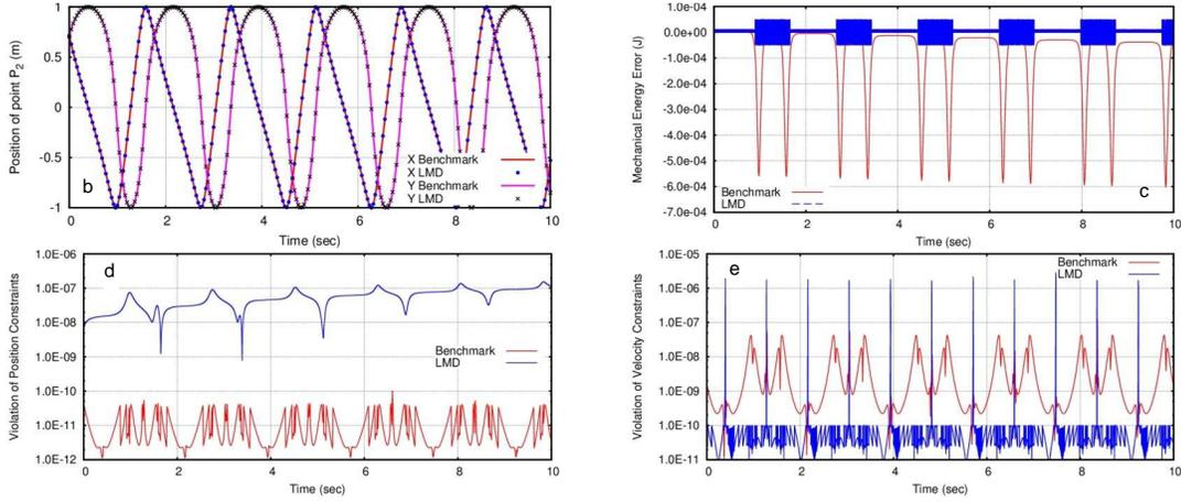
**Fig. 2.** (a) Mechanical model of a slider-crank mechanism, (b)  $x$  and  $y$  coordinates of point  $P_2$ , (c) mechanical energy, (d) violation of position and (e) violation of velocity constraints.
