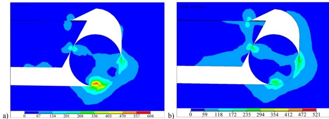
Figure 5. Equivalent von Mises stresses (MPa) in the contact area of the pipe and fastening for the different values of friction coefficient: a)  $f = 0.4$ ; b)  $f = 0.06$
