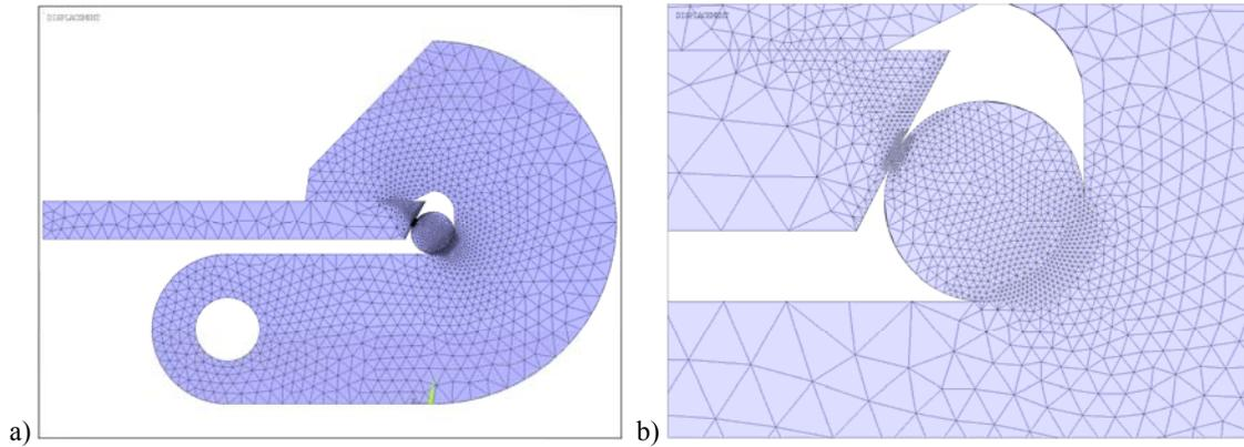
Figure 4. Finite element model: a – full model; b – elements contact areas
