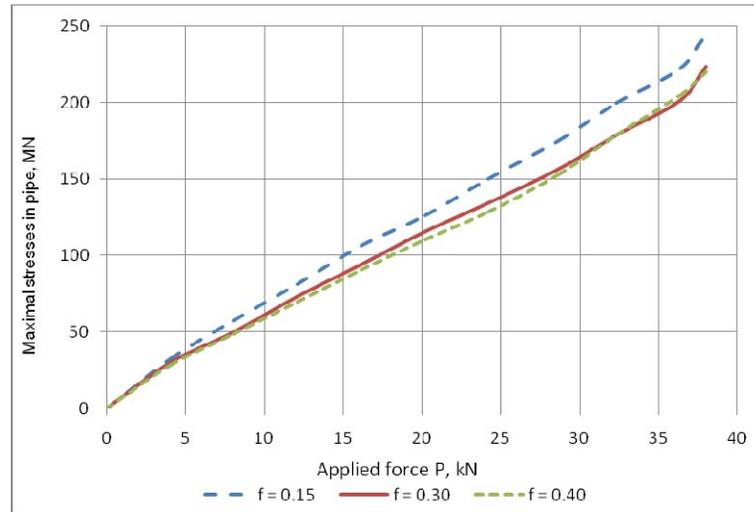
Figure 7. The dependence of the maximal stresses in the pipe on the applied force  $T$
