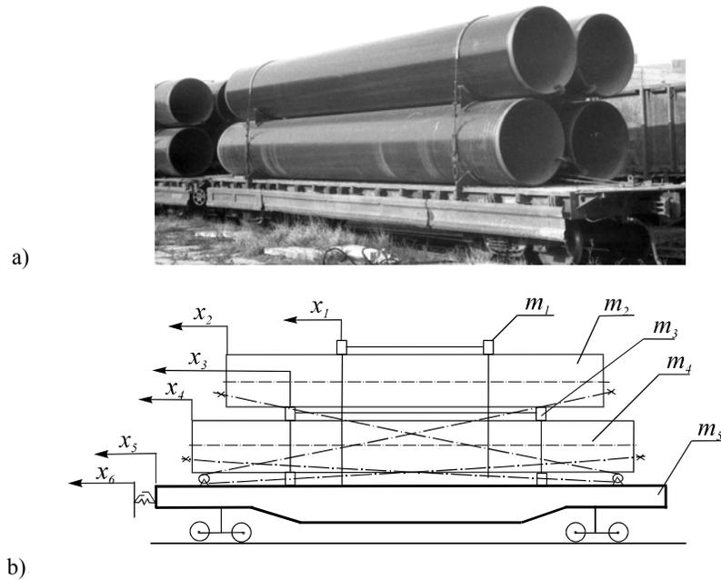
Figure 1. A flatcar with pipes: real fastening (a) and normative scheme (b)
