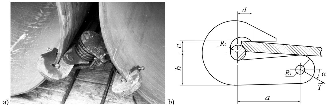
Figure 2. Self-aligning devices for fixing pipes: photo (a) and scheme (b)
