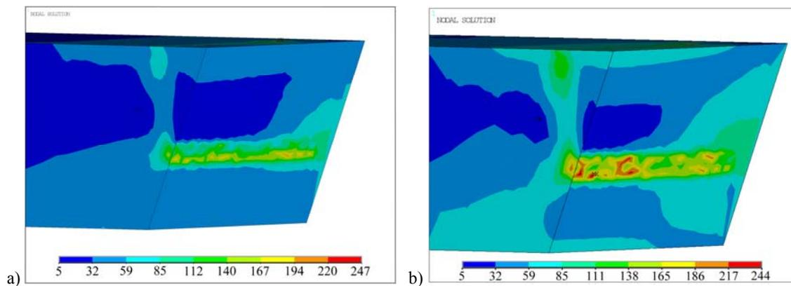
Figure 6. Equivalent von Mises stresses (MPa) in the insert-pipe contact point for the different values of friction coefficient: a)  $f = 0.4$ ; b)  $f = 0.06$
