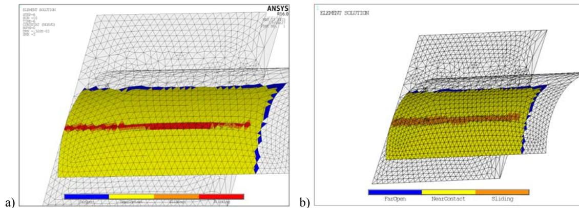
Figure 8. The insert-pipe contact status for the different values of friction coefficient: a)  $f=0.4$ ; b)  $f=0.06$
