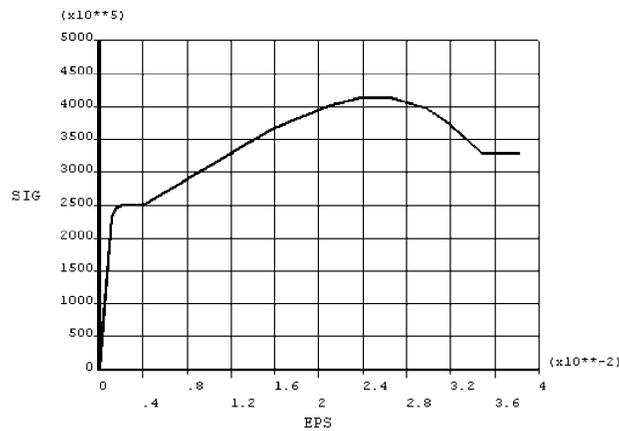
Figure 3. Diagram for the pipe material stretching
