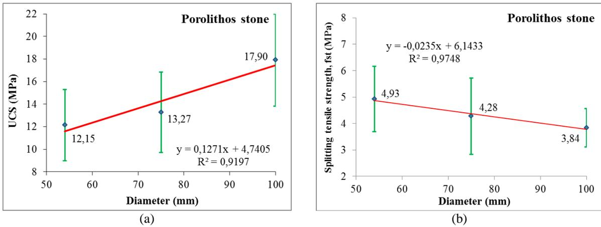
Figure 8. (a) Uniaxial compression strength and (b) Splitting tensile strength of Porolithos stone in correlation with the diameter.
