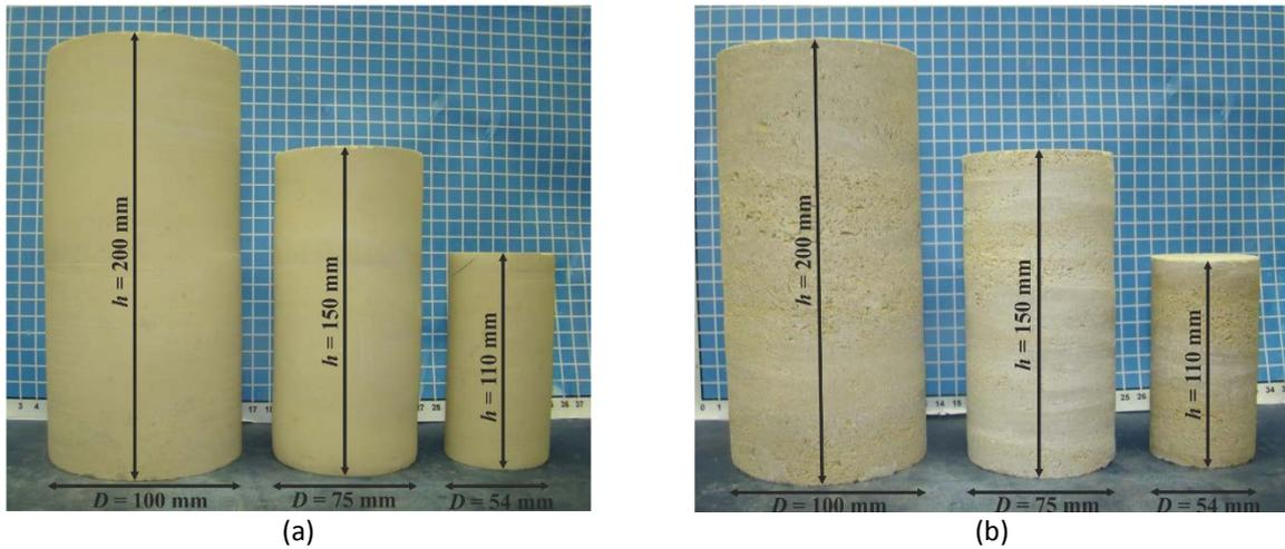
Figure 5. A series of cylindrical specimens with different diameters for (a) Alfás stone and (b) Porolithos stone.
