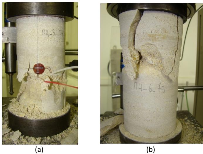
Figure 10. Typical mode of fracture in Porolithos cylindrical specimens.
