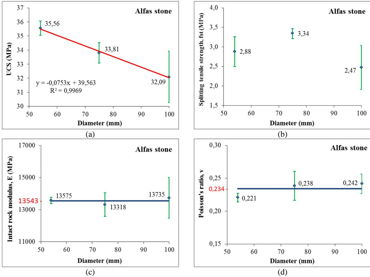
Figure 7. (a) Uniaxial compression strength, (b) Splitting tensile strength, (c) Intact rock modulus and (d) Poisson's ratio of Alfaf stone in correlation with the diameter.
