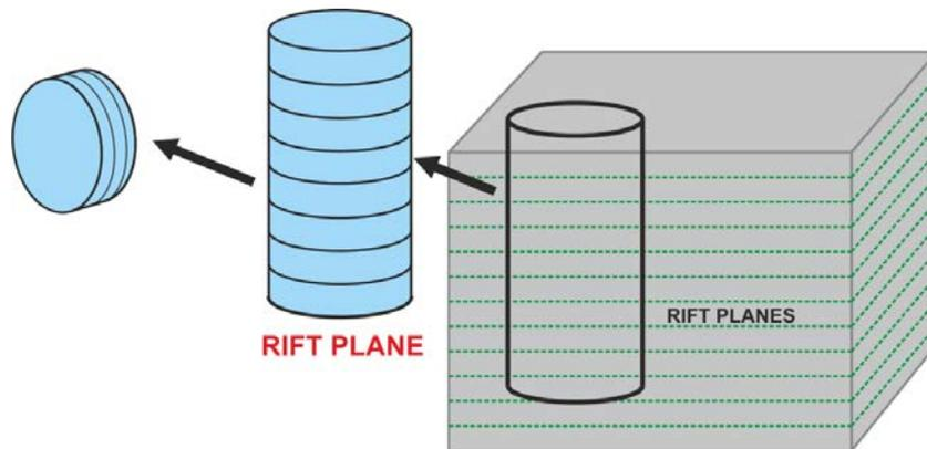
Figure 4. The orientation of the Porolithos specimens. The plane perpendicular to the symmetry axis of the cylindrical specimens is parallel to the plane of transverse isotropy (rift planes).
