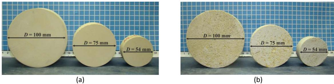
Figure 6. A series of discs with different diameters for (a) Alfás stone and (b) Porolithos stone.
