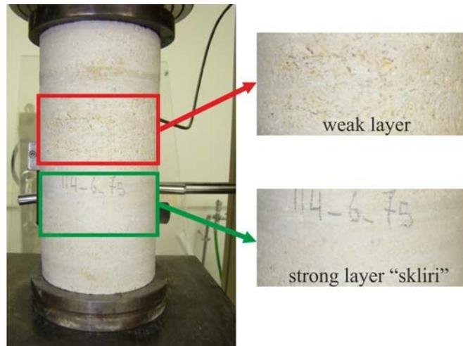
Figure 1. Horizons with different mechanical characteristics evident in a cylindrical specimen of the Porolithos stone.
