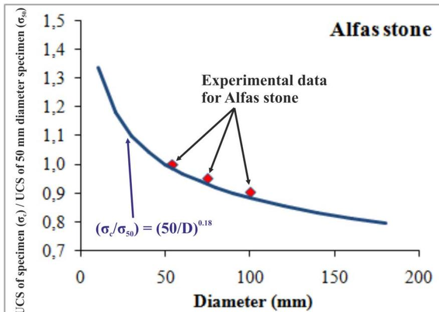
Figure 12. Relationship between UCS and specimen size plotted as dimensionless values [24].
