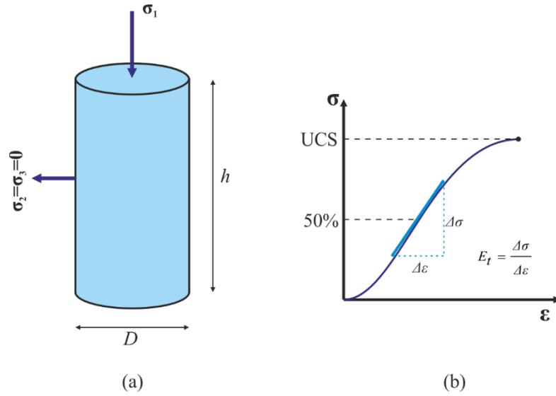
Figure 2. (a) Uniaxial compression test. (b) Stress-strain curve and the calculation of the tangent intact rock modulus.
