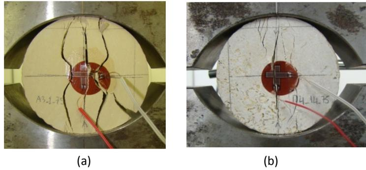
Figure 11.(a) Center primary fracture plane with typical secondary fractures in Alfás circular disc. (b) Center primary fracture plane in Porolithos circular disc.
