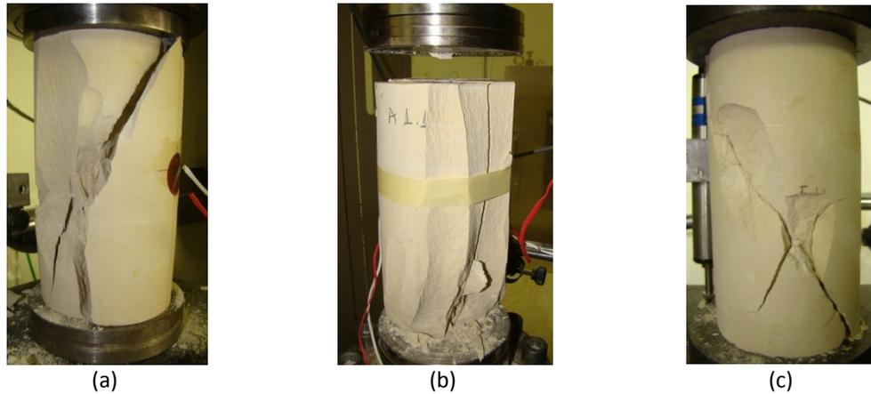
Figure 9. Typical crack patterns in Alfas cylindrical specimens. (a) Shear plane failure (b) Axial splitting failure (c) Failure on conjugate shear planes.
