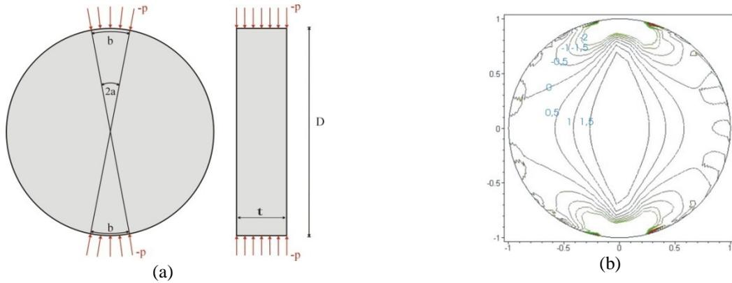
Figure 3. (a) Load configuration of the Brazilian test, (b) Distribution of the horizontal Stress Concentration factor  $q_{xv} = \sigma_{xv} / (pa/\pi)$  calculated from the theory of elasticity [21].
