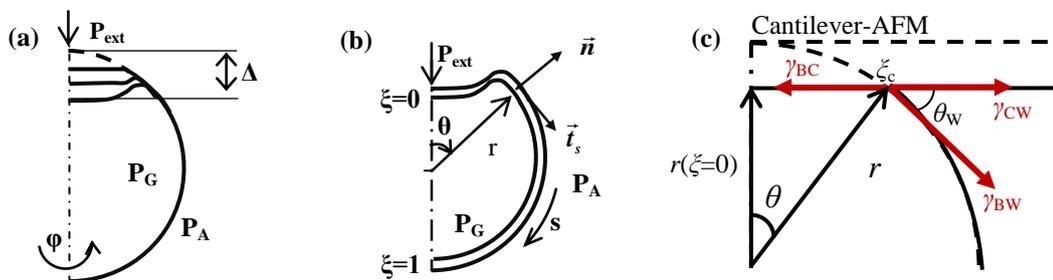
Figure 2. (a) Deformed bubble subject to an increasing static point load, (b) lagrangian representation, (c) schematic description of contact between the microbubble and the AFM
