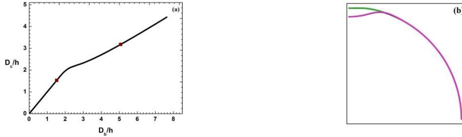
Figure 6.(a) Cantilever displacement versus shell displacement and (b) Microbubble in deformed configuration for  $d/h=1.5$  and  $5$ , corresponding on red dots of (a), both for a polymeric microbubble.
