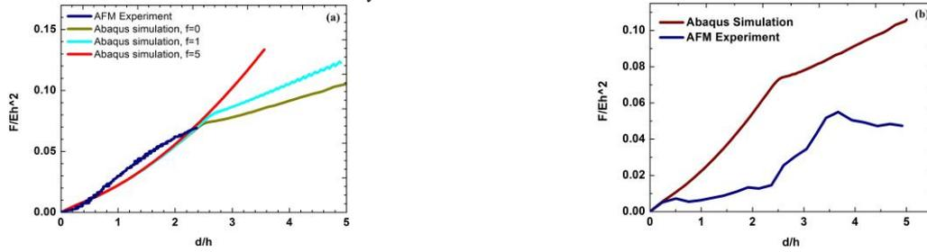
Figure 5. Force-deformation curves obtained with Abaqus against experimental data for (a) a polymeric microbubble ( $R_0=1.3 \mu\text{m}$ ;  $\chi=212 \text{ N/m}$ ) [3] and (b) a phospholipid shell ( $R_0=1.82 \mu\text{m}$ ;  $\chi=0.085 \text{ N/m}$ ) [2]
