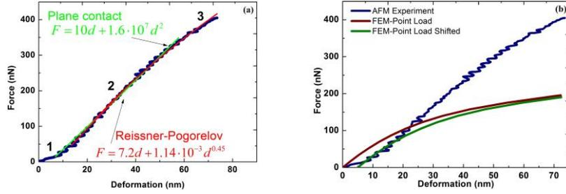
Figure 1 (a) Asymptotic fitting in f-d curve of a polymeric microbubble [3], (b) Comparison between experimental [3] and FEM results for a point load on a polymeric microbubble
