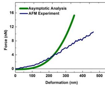
Figure 3.  $F$ - $d$  plot of based on equation (22) against experimental [2] AFM data for a lipid microbubble with  $R_o=1.82 \mu\text{m}$ ;  $\chi=0.085 \text{ N/m}$ ;  $W_s=10^{-5} \text{ N/m}$
