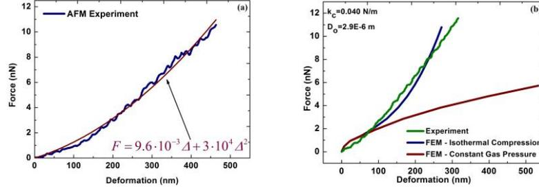
Figure 4. (a) Asymptotic fitting in f-d curve for a lipid microbubble [2], (b) Comparison between experimental [2] and FEM results for a microbubble covered with phospholipid
