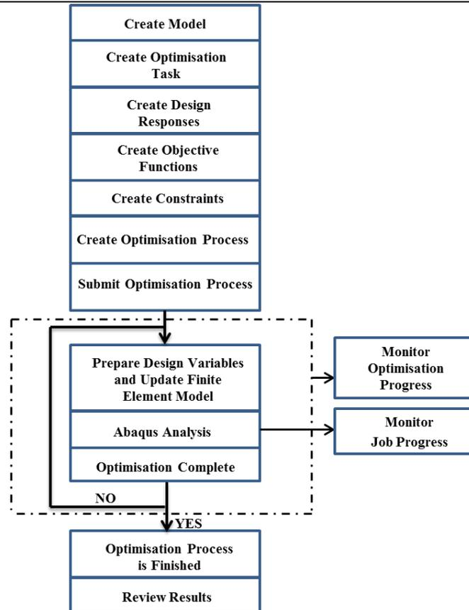
Figure 2. Optimisation Process in Abaqus
