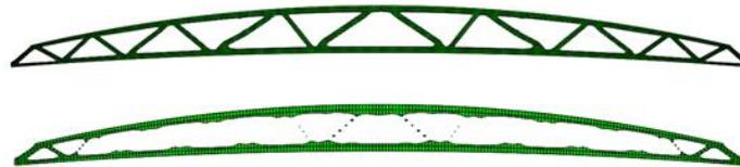
Figure 5. Last design cycle of optimisation process for fine and coarse mesh respectively
