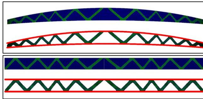
Figure 8. Optimised truss topologies with stringers on the top and bottom chord
