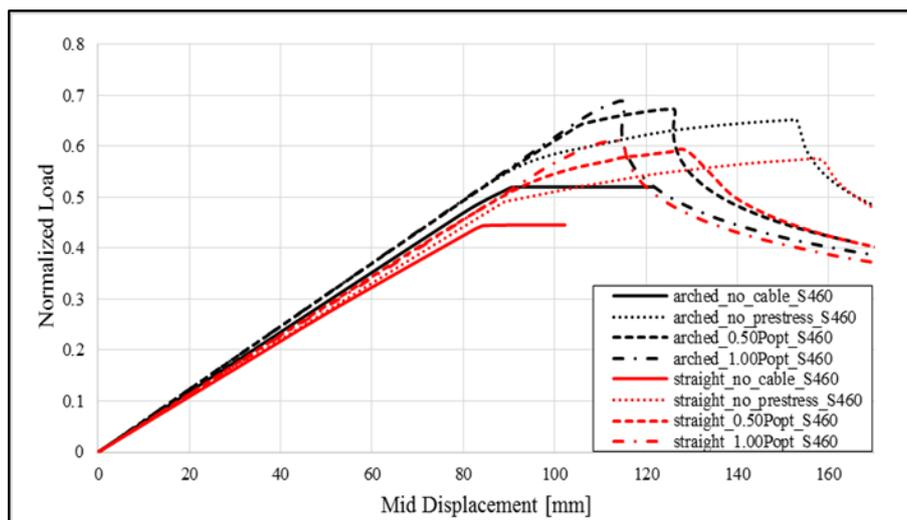
Figure 11. Normalised load vs midspan displacement for S460 trusses
