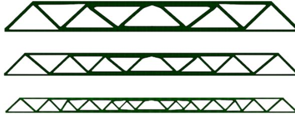
Figure 7. Optimised trusses for H/L=0.10, 0.075, 0.05 respectively
