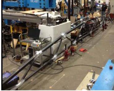
Figure 4. HSS trusses to be tested at Imperial College
