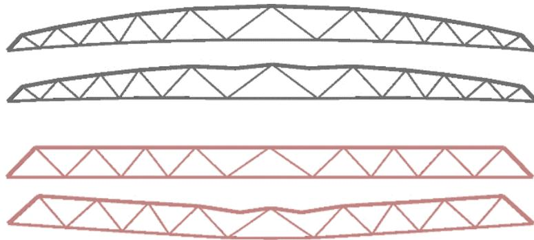
Figure 10. Typical deformed shapes for the two truss configurations
