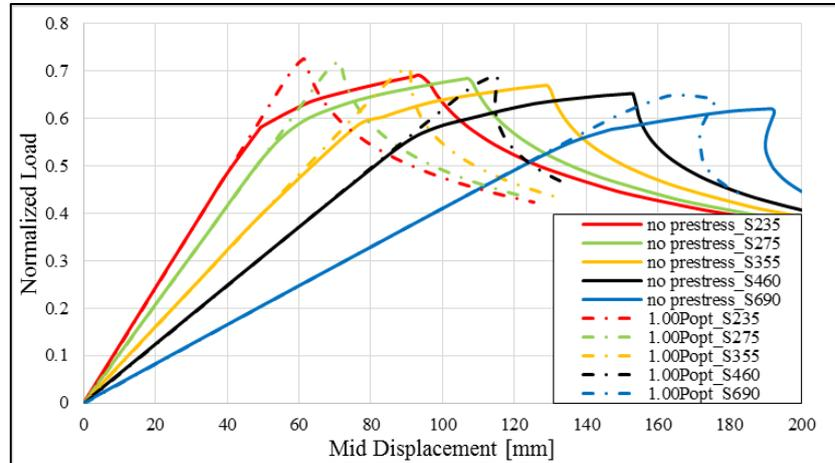
Figure 13. Normalised load vs midspan displacement for zero and  $1.00P_{opt}$  prestress
