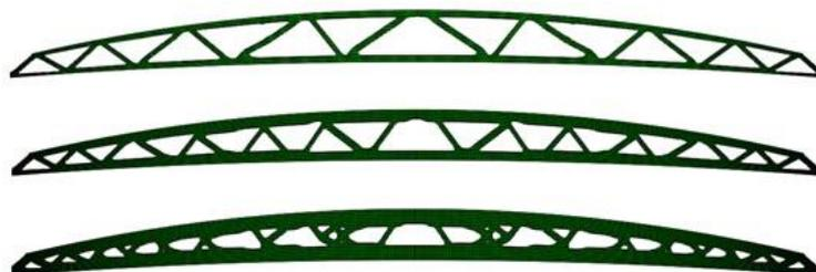
Figure 6. Influence of the volume constraint -  $V_{\text{final}}/V_{\text{initial}}$  0.3, 0.5, 0.7 respectively
