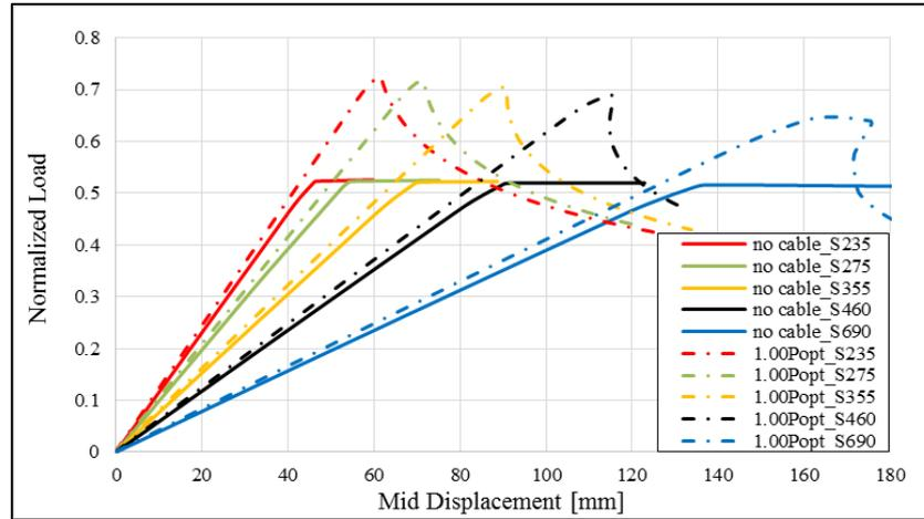
Figure 12. Normalised load vs midspan displacement for varying steel grade
