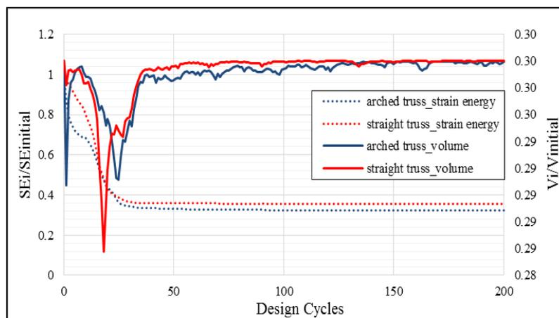
Figure 9. Objective function and volume constraint vs optimisation design cycle
