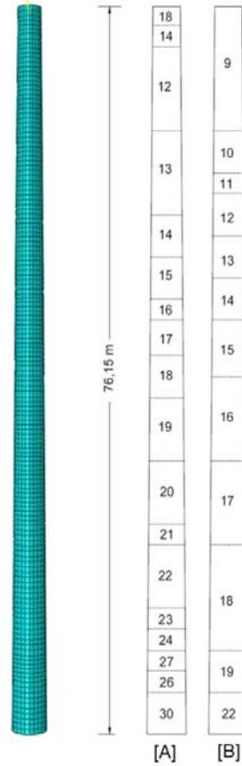
Figure 2. Shell thicknesses of investigated towers [A] and [B].
