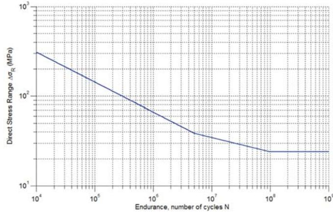
Figure 9. Direct Stress Range over number of cycles for the structural detail investigated
