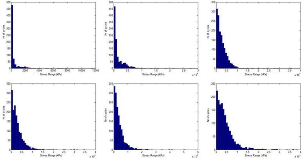
Figure 6. Tower [B] stress range histograms for variable mean wind speeds
