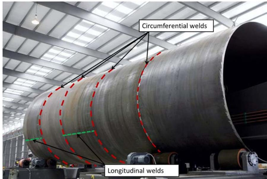
Figure 1. Position of longitudinal and circumferential welds (Source: <http://www.gosanangelo.com>)
