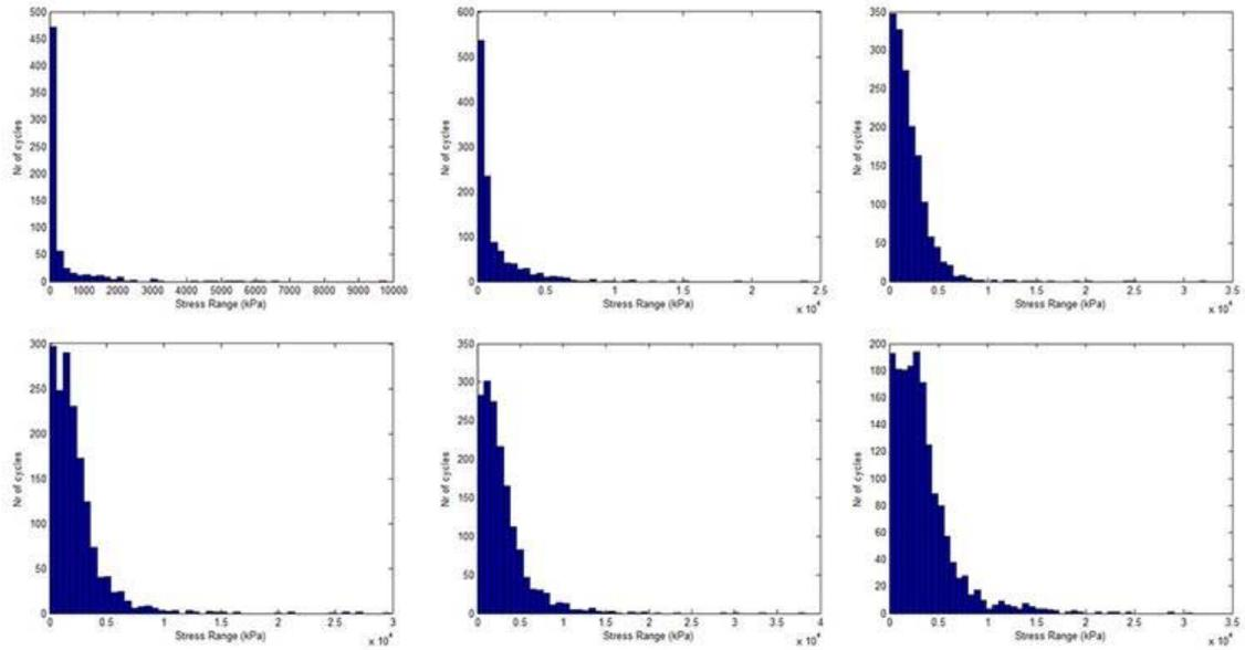
Figure 5. Tower [A] stress range histograms for variable mean wind speeds
