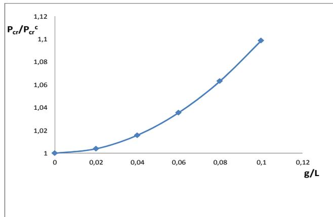
Fig.10. Variation of the dimensionless buckling load  $P_{cr}/P_{cr}^c$  versus  $g/L$  for the fig. 9..
