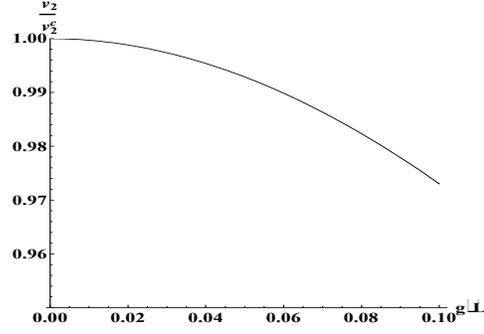
Fig. 6. Deflection versus  $g/L$  of the simply supported gradient elastic beam of Fig.5
