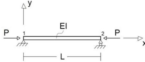
Fig.9. Geometry of a simply supported gradient elastic beam under an axial compressive load
