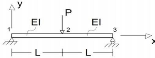
Fig.5 Geometry and loading of a simply supported gradient elastic flexural beam
