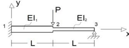
Fig.7. Geometry and loading of a fixed-hinged gradient elastic beam composed of two members with different cross-sections
