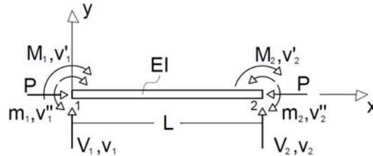
Fig.4. Matrix convention for generalized nodal forces and displacement of gradient elastic flexural beam element with a constant compressive axial force
