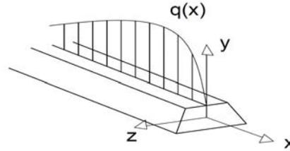
Fig. 1 Geometry and loading of a prismatic beam in bending
