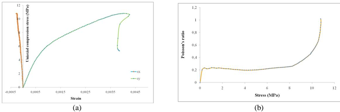
Figure 5. (a) Axial stress vs axial and lateral strain (b) Variation of Poisson's ratio with the axial stress.
