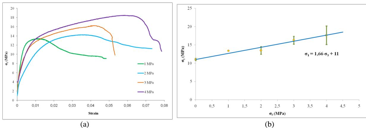
Figure 6. (a) Stress – strain curves for different lateral stresses (b) Confined uniaxial compression strength vs lateral stresses.
