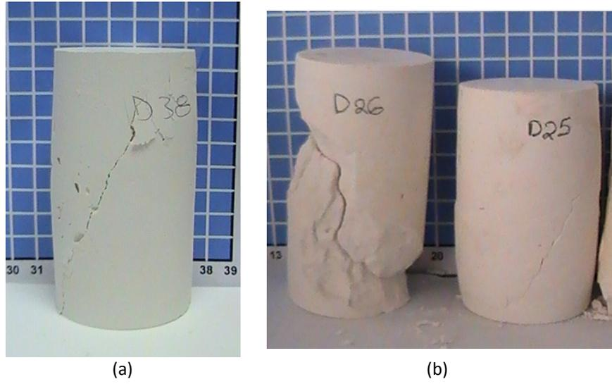
Figure 7. Typical crack patterns in pozzolanic mortar cylindrical specimens in (a) uniaxial compression test and (b) triaxial compression test.
