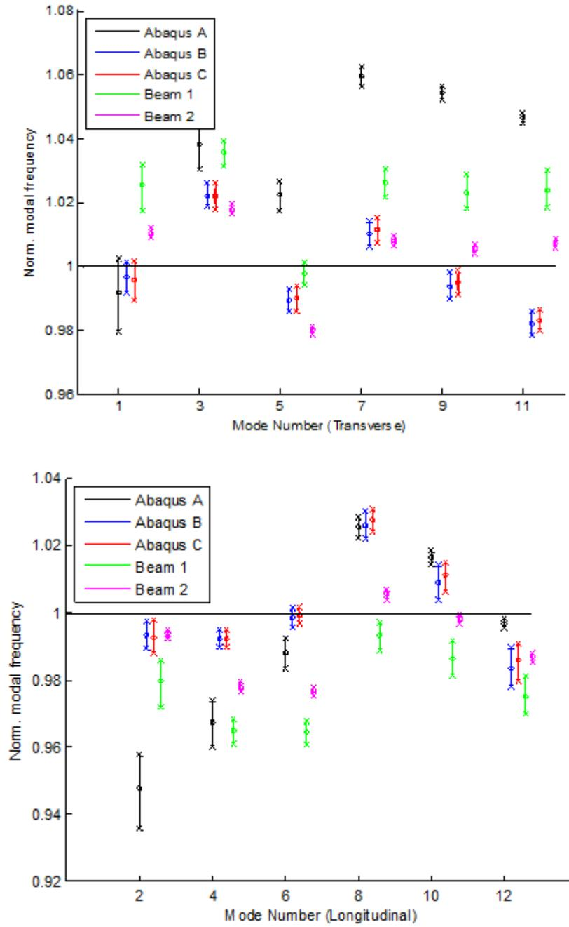
Figure 3: Uncertainty propagation to the output modal frequencies. Abaqus A  $\equiv$  FE-1, B  $\equiv$  FE-2, C  $\equiv$  FE-3, Beam 1  $\equiv$  Beam - Fixed, Beam 2  $\equiv$  Beam - Flex
