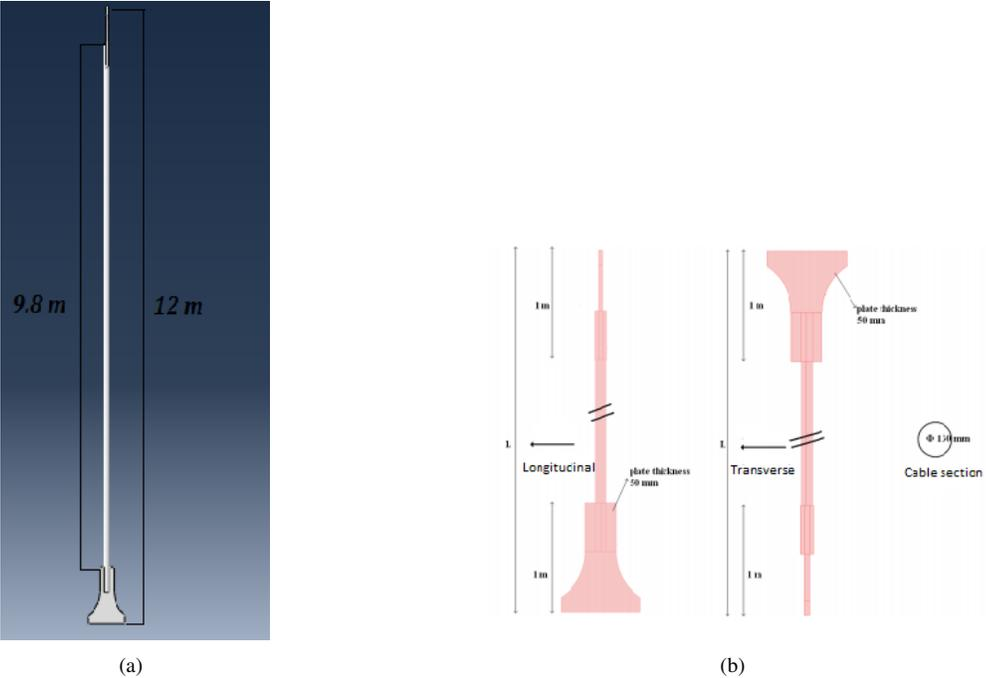
Figure 2: (a) The geometry of hanger 3, (b) The geometry of the plates connecting the circular hanger to the arch and the deck of the bridge
