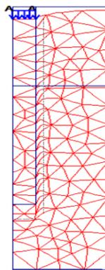
Figure 5. Deformed shape of the soil-pile due to the vertical load which is subjected at the head of the pile.
