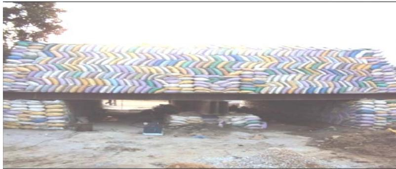
Figure 1. Single pile subjected to vertical load in the field test [4].
