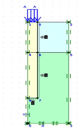
Figure 2. The two-dimensional built model with applied vertical load in FEM code.
