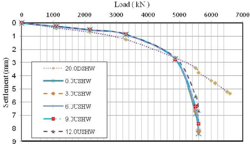
Figure 11. Load - Settlement curves for undrained soil with respect to variation of water level, for the pile (with  $L=15 m, D=1 m$ ).
