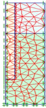
Figure 3. Discretizing the model using a set of 15-node triangle elements and the interface elements of between soil and pile.
