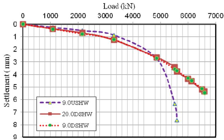
Figure 9. Load-settlement curves for the pile with  $L=15m$  and  $D=1m$  and  $H_w=9m$ .
