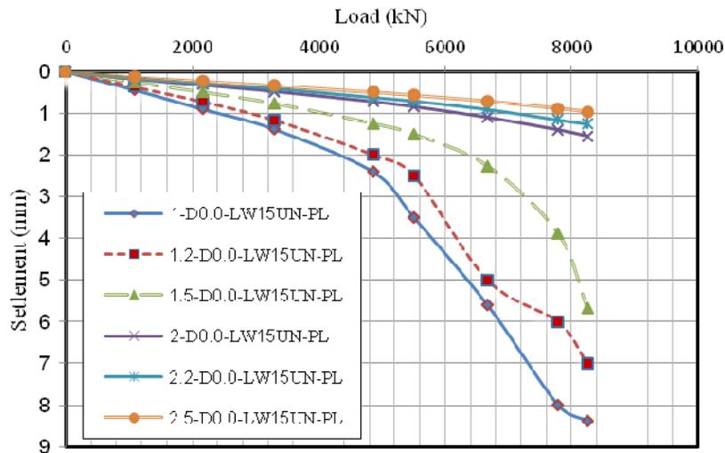
Figure 12. Load - Settlement curves for undrained soil with respect to variation of pile diameter ( $Hw = 0 m$ , undrained soil).
