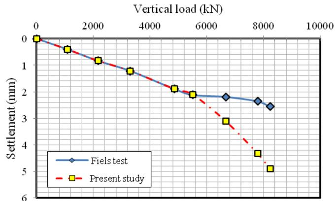
Figure 4. The results of the Load-Settlement Curve for the pile regarding field study [4] and the present study.
