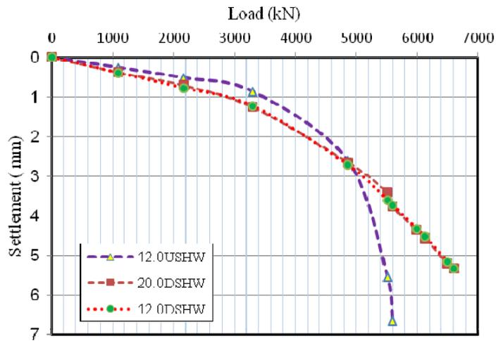
Figure 10. Load-settlement curves for the pile with  $L=15m$  and  $D=1m$  and  $H_w=12m$ .
