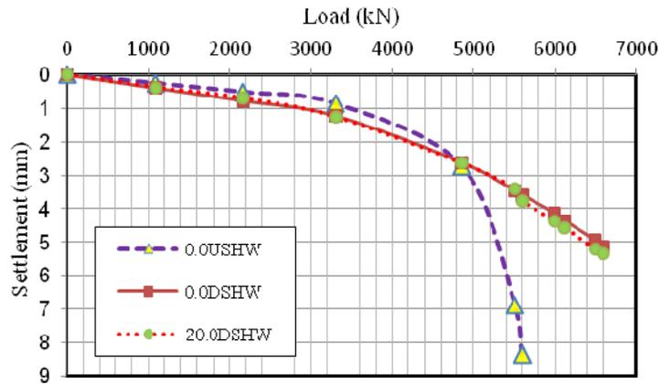
Figure 6. Load-settlement curves for the pile with L=15m and D=1m and Hw=0m.
