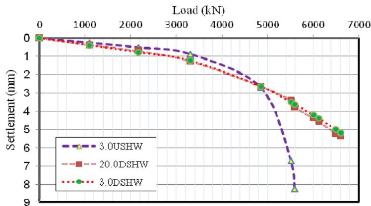
Figure 7. Load-settlement curves for the pile with L=15m and D=1m and Hw=3m.
