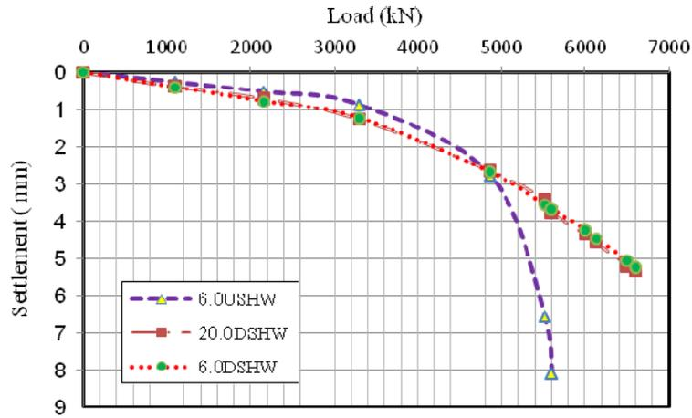
Figure 8. Load-settlement curves for the pile with  $L=15m$  and  $D=1m$  and  $H_w=6m$ .
