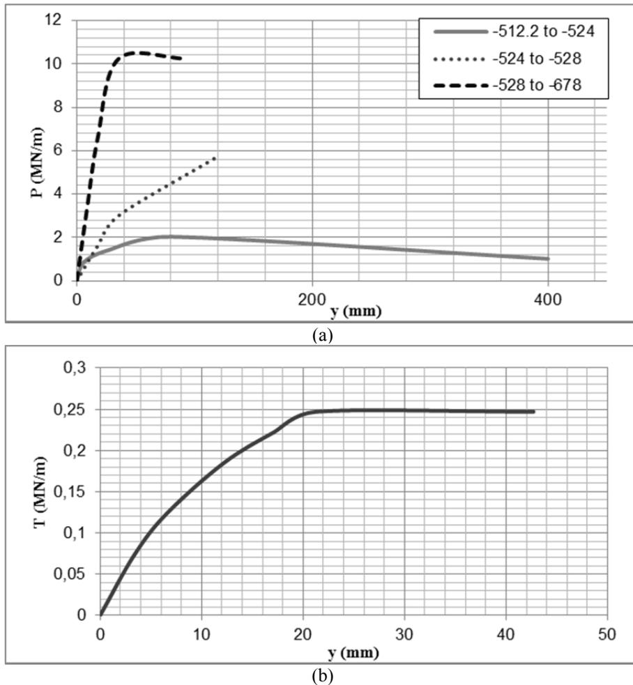
Figure 3. Soil response curves for the (a) horizontal and (b) vertical direction.
