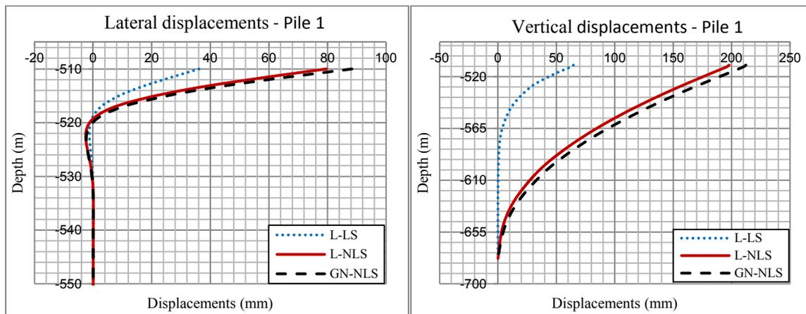
Figure 4: Lateral – Vertical displacements of Pile 1.
