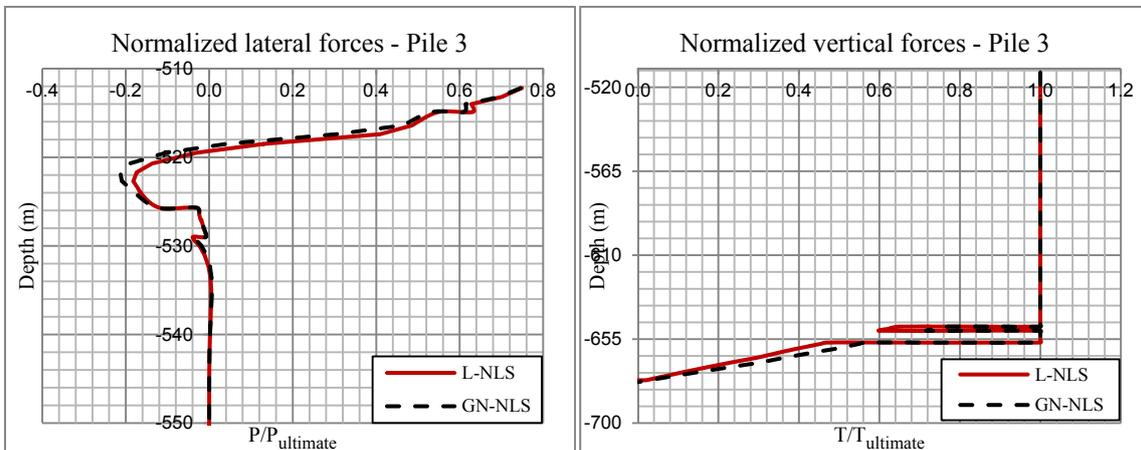
Figure 9: Soil reactions under Pile 3.
