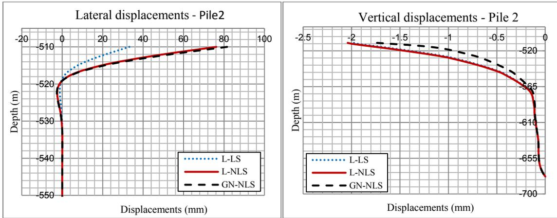
Figure 5: Lateral - Vertical displacements of Pile 2.
