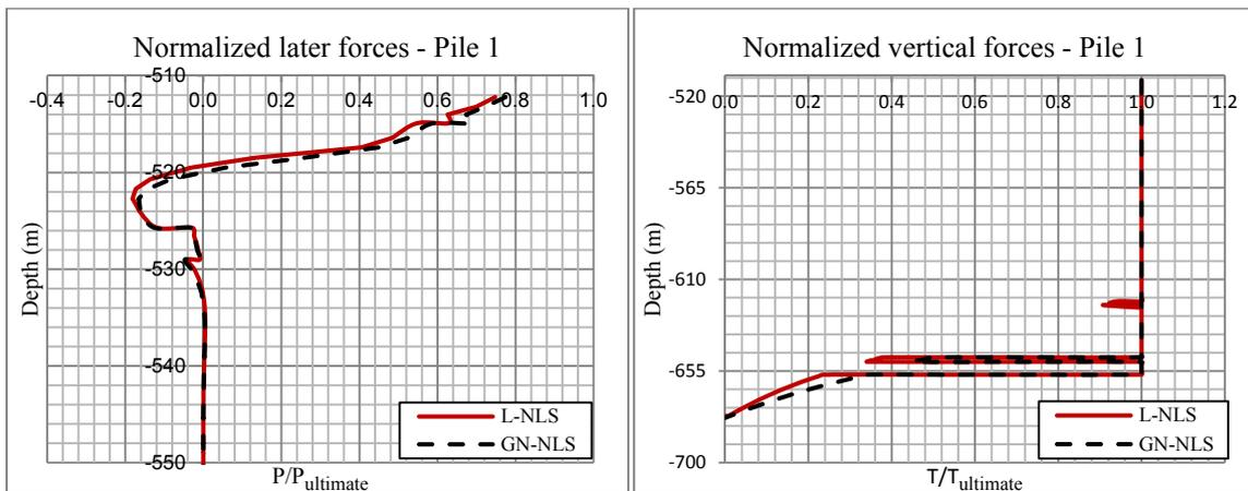
Figure 7: Soil reactions under Pile 1
