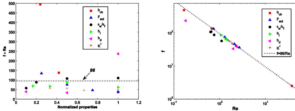
Figure 4. a) The modification factor (Eq. (9)) for various nano-flow conditions. Each parameter on the horizontal axis is normalized to its maximum value for presentation reasons and b)  $f$  vs.  $Re$  fully logarithmic diagram.
