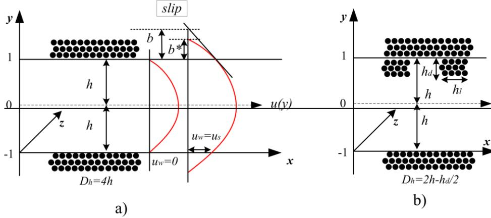
Figure 1. a) Atomistic model of Poiseuille flow at the nanoscale. Velocity profiles with slip and no-slip are shown. b) Atomistic model of flow in rough-wall nanochannels, where  $h_l$  is the length and  $h_d$  is the height of roughness rectangular protrusions.  $D_h$  is the hydraulic diameter.
