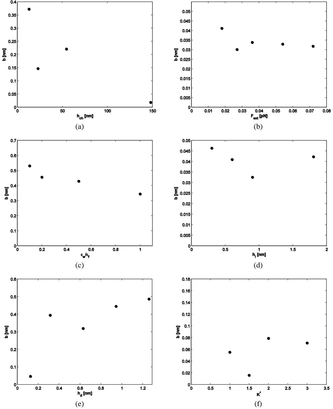
Figure 3. Slip length,  $b$ , vs. a) channel width, b) magnitude of the external force, c) wall wettability ratio, d) roughness length, e) roughness height and f) spring constant value. Simulation conditions are the same as the respective cases in Fig. 2.
