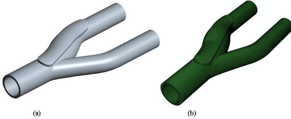
Figure 2: Patched carotid artery with 6mm ICA internal diameter: (a) Schematic representation of the 3D model, (b) FE mesh.
