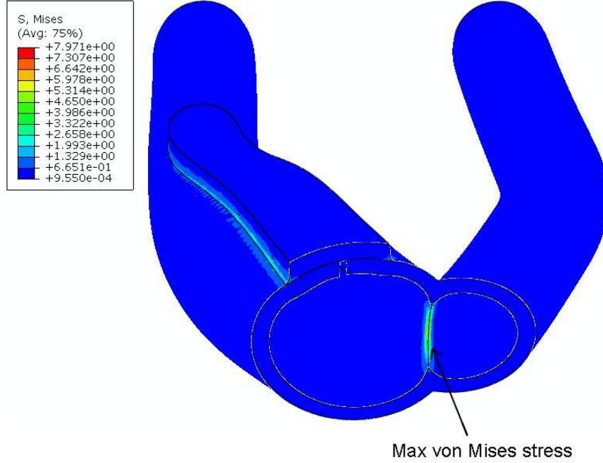
Figure 4: Carotid artery with CCA internal diameter 6mm after unloading and reloading with a twofold increase of systolic pressure. Maximum von Mises equivalent stress appears in the bifurcation.
