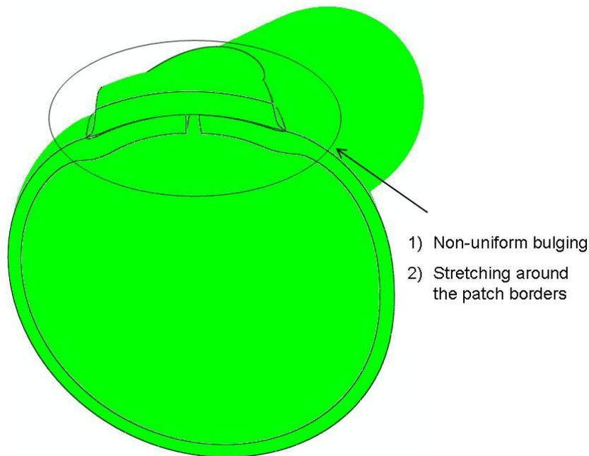
Figure 6: Deformed configuration ( $2\times$ ) of the carotid artery with CCA internal diameter 6mm and patch elastic modulus  $E = 40$  MPa after unloading and reloading with a twofold increase of systolic pressure.
