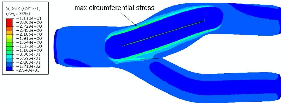
Figure 5: Carotid artery with CCA internal diameter 6mm after unloading and reloading with a twofold increase of systolic pressure. Maximum circumferential stress appears in the connecting region of the patch with the arterial wall.
