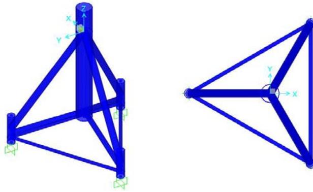
Figure 10: Simulation of the fixed tripod in SAP2000
