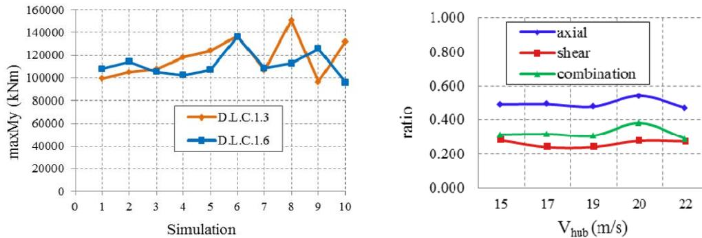
Figure 5: Maximum value of bending moment  $M_y$  for DLC 1.3 and DLC 1.6 for  $V_{hub}=20\text{m/s}$  and exploitation ratio of the most unfavorable output station for different velocities  $V_{hub}$
