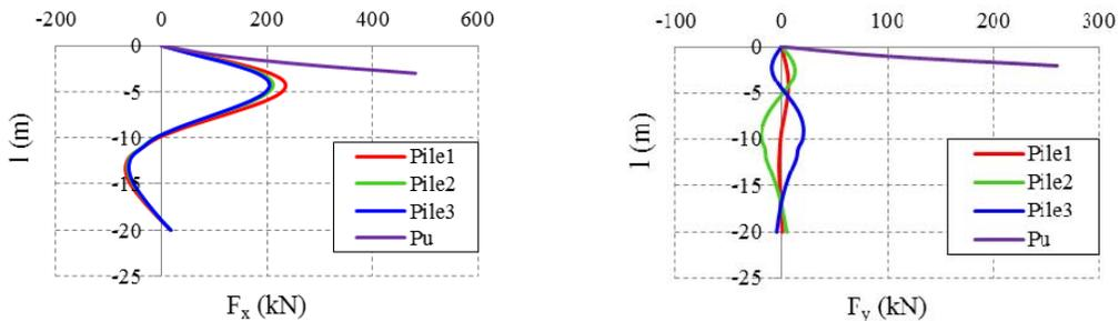
Figure 14: Spring reactions  $F_x$  (kN) and  $F_y$  (kN) for the three piles
