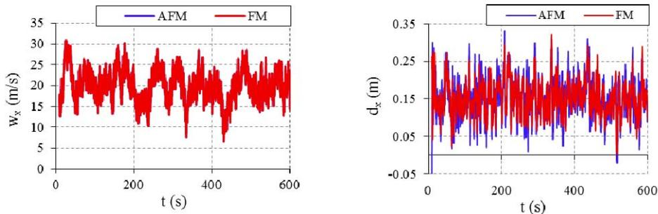
Figure 9: Wind speed  $w_x$  (m/s) time series and deformation  $d_x$  (m) at the top of the turbine for Apparent Fixity (AFM) and Fixed Model (FM)
