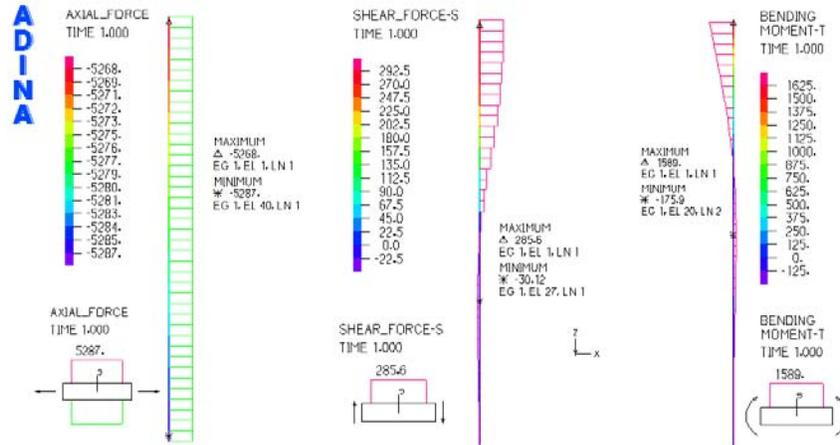
Figure 13: Pile 1- Axial, Bending and Shear Forces for DLC 1.3-MaxMy-L=20m
