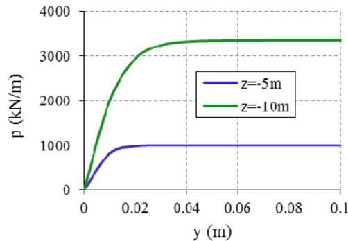
Figure 2: Load- displacement curves for depths  $z=-5m$  and  $z=-10m$
