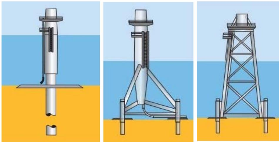
Figure 1: Monopile, Tripod and Jacket Foundation [Source: EWEA]
