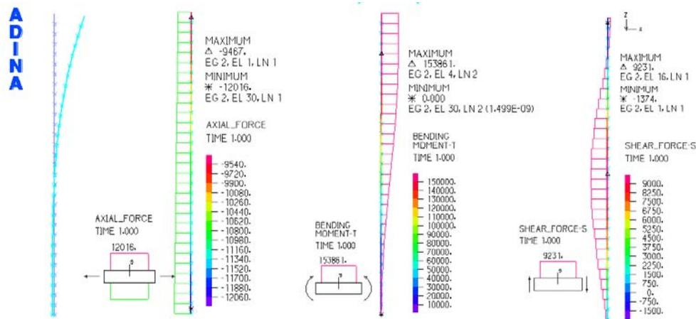
Figure 6: Deformed shape, axial and shear forces and bending moments for DLC 1.3-MaxMy-L=30m
