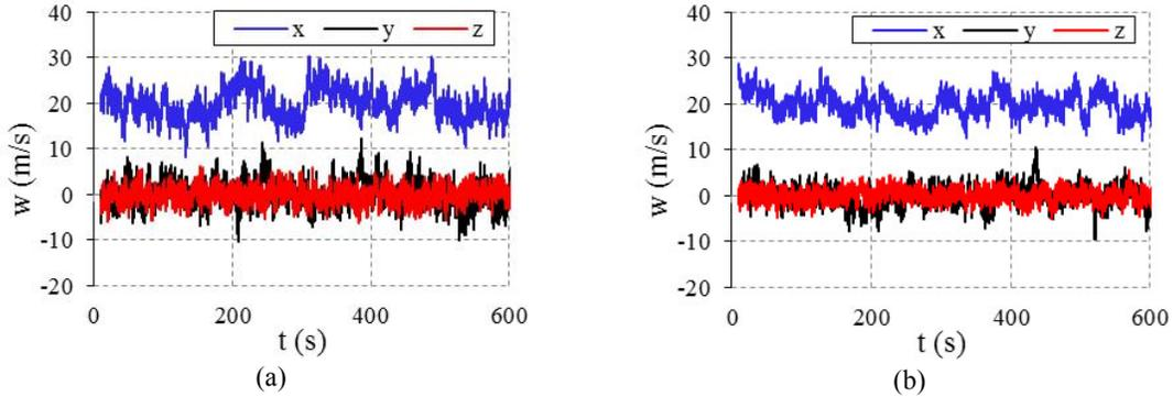
Figure 3: Wind velocity (m/s) time histories in three directions for DLCs 1.3(a) and 1.6a(b) with  $V_{hub}=20\text{m/s}$
