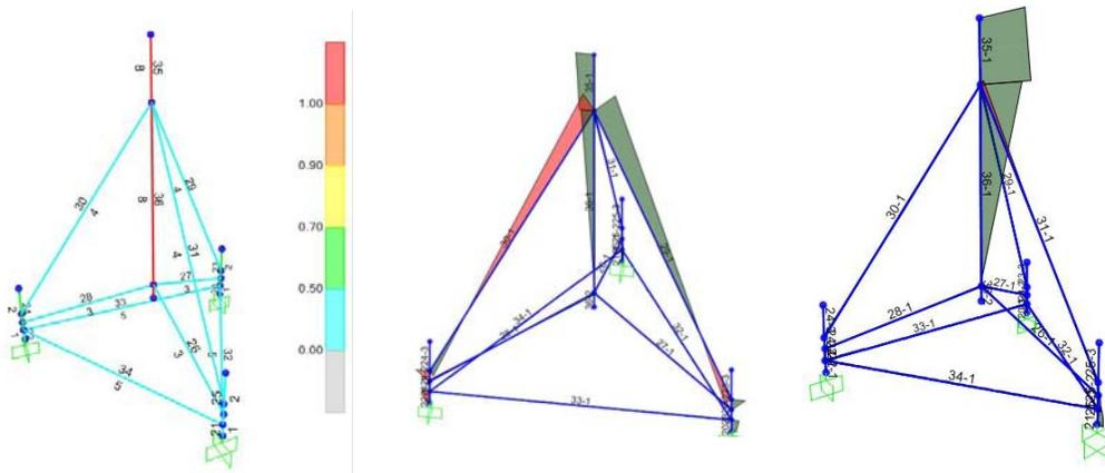
Figure 11: Ratios of exploitation and Bending Moments  $M_x$ ,  $M_y$  for the worst loading case
