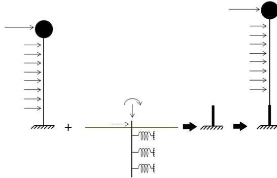
Figure 8: Procedure of analysis of the offshore wind turbine and determination of the AFM
