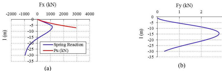
Figure 7: Spring reactions  $F_x$  (kN) and  $F_y$  (kN)
