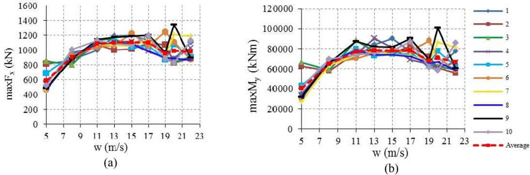
Figure 4 : DLC 1.3-Maximum actions  $M_y$ ,  $F_x$  at the transition piece level for different mean wind speeds  $V_{hub}$  (m/s) and for 10 simulations
