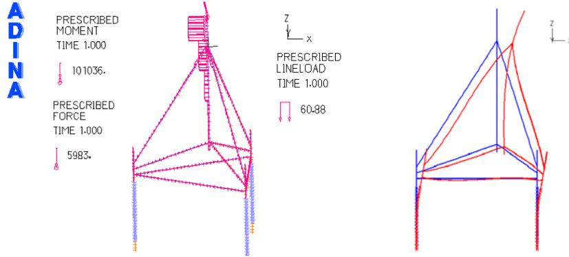
Figure 12: Modeling in ADINA and deformed geometry
