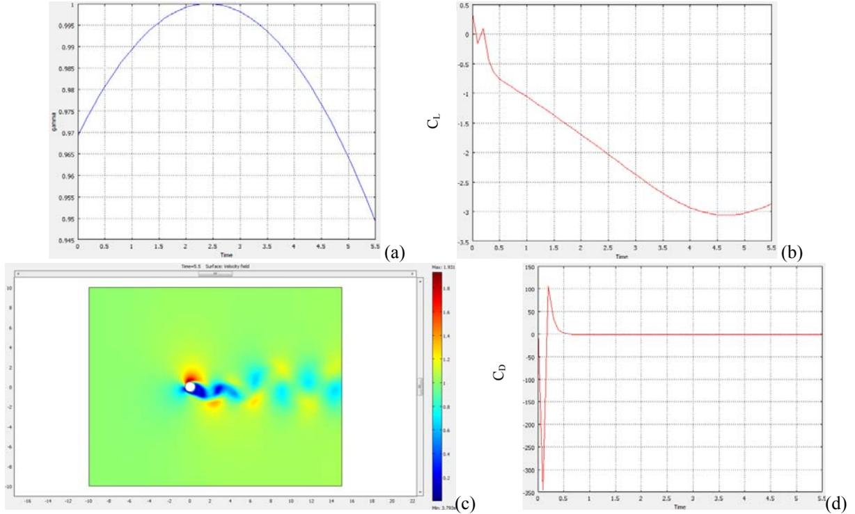
Figure 4: Optimization results for the 2-dof case A: optimal control action (a), resulting lift coefficient (b), velocity field profile after 5.5 time units (c) and temporal profile of the corresponding drag coefficient (d).
