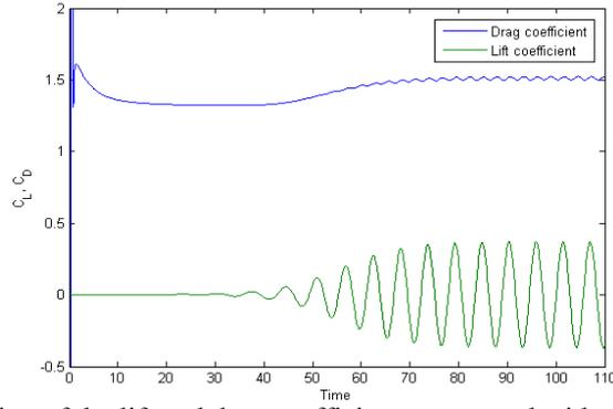
Figure 2: Time evolution of the lift and drag coefficients computed with a full-scale CFD model.
