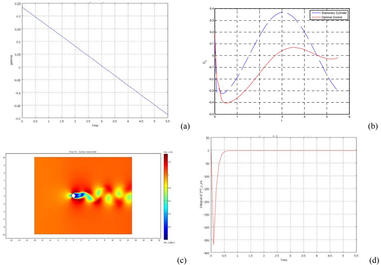
Figure 3: Optimization results for the 3-dof case: optimal control action (a), resulting lift coefficient (b), velocity field profile after 5.5 time units (c) and temporal profile of the corresponding drag coefficient (d).
