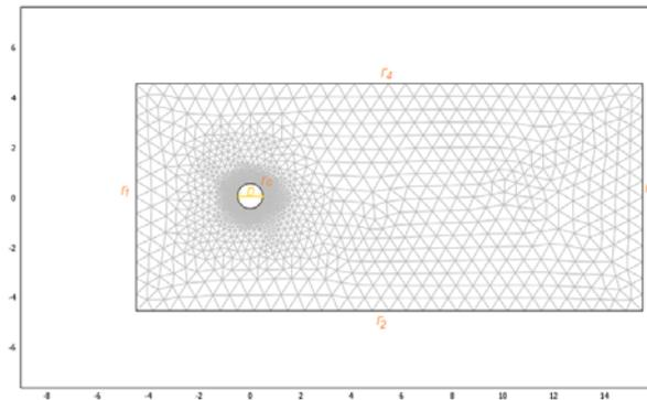
Figure 1: The computational domain for the benchmark problem and the discretization mesh.
