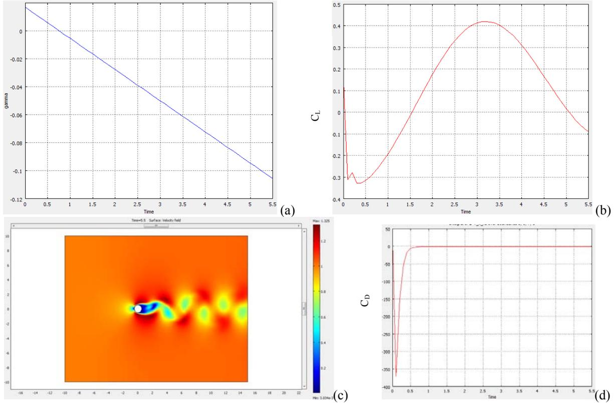
Figure 5: Optimization results for the 2-dof case B: optimal control action (a), resulting lift coefficient (b), velocity field profile after 5.5 time units (c) and temporal profile of the corresponding drag coefficient (d).
