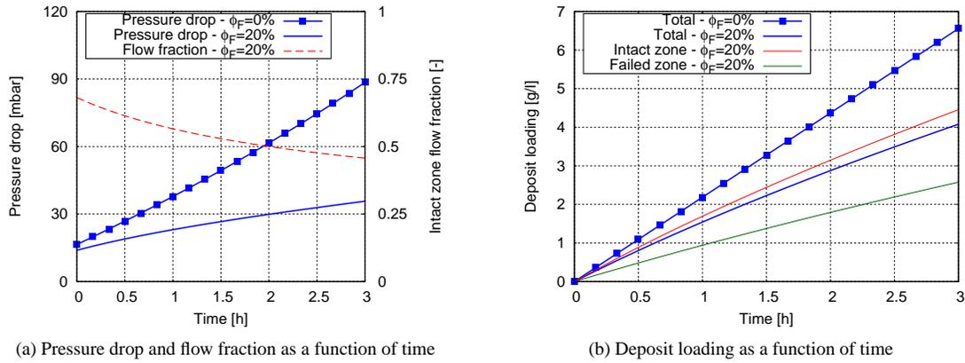
Figure 5: Pressure drop, flow fraction and deposit loading of a filter with 20% failure level as a function of time.
