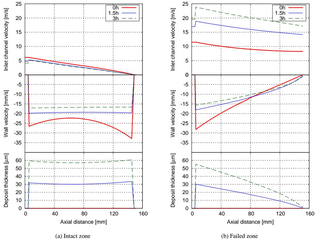
Figure 4: Velocity and deposit thickness profiles in a filter with 20% failure level.
