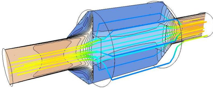
Figure 2: Streamlines and velocities in a filter with 20% failure level.
