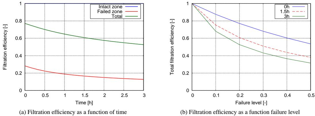
Figure 6: Filtration efficiency as a function of time and failure level.
