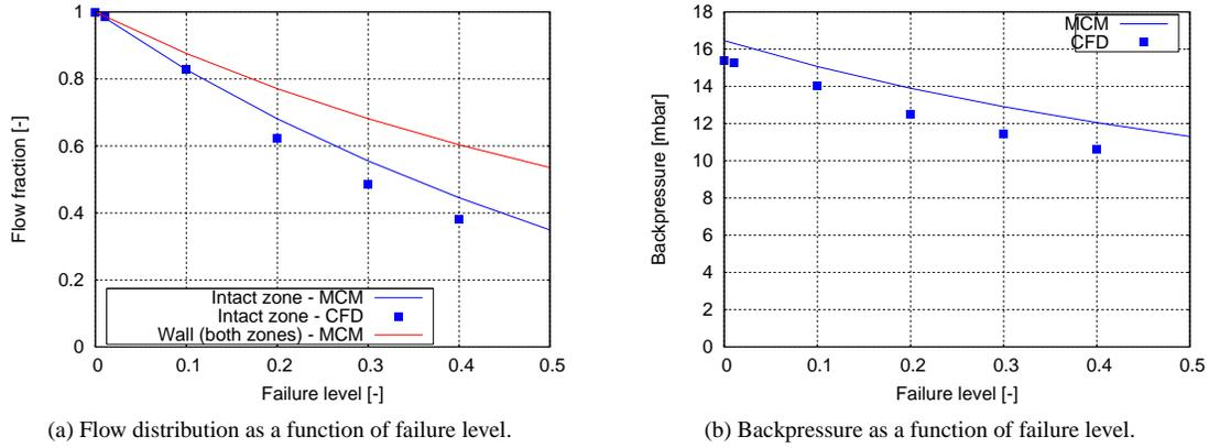
Figure 3: Flow performance at clean state as a function of failure level.
