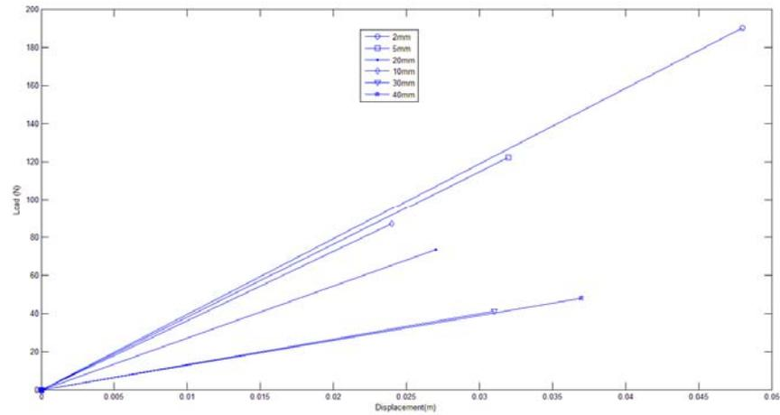
Figure 10: The Load Displacement curves of pure tensile numerical tests.
