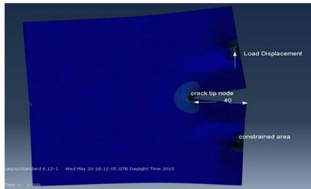
Figure 9: Finite Element model of a typical length 40mm subjected in pure tensile load.
