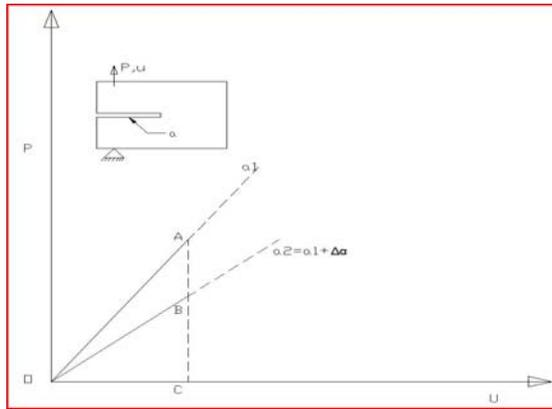
Figure 2: Load displacement response of a cracked plate from length  $a_1$  to  $a_2$  under 'fixed grips' conditions along AB
