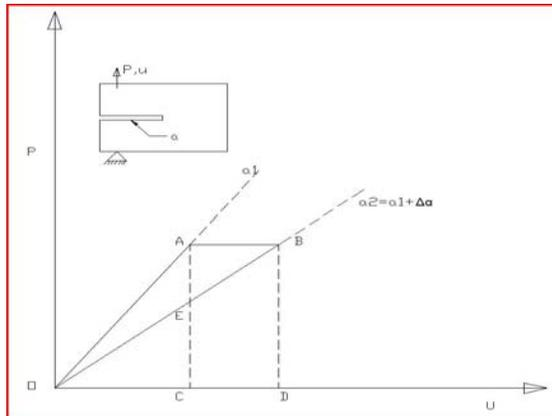
Figure 3: Load displacement response of a cracked plate for length  $a_1$  to  $a_2$  under 'fixed grips' conditions along AB
