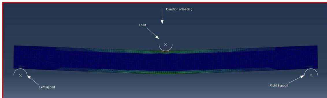
Figure 6: Solution of the Finite element analysis of the uncracked sandwich beam
