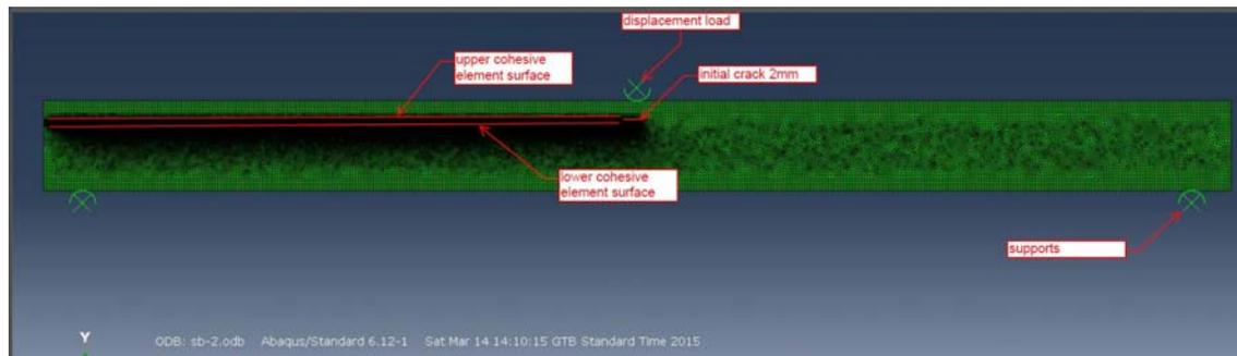
Figure 11: The Cohesive Finite Element Model.
