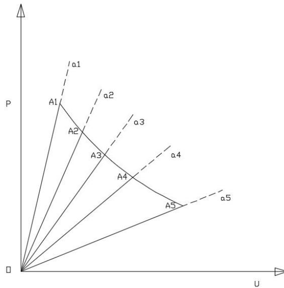
Figure-4: Load displacement response of a cracked plate for propagation of a crack from an initial length  $a_1$  to a final length  $a_5$  under load - displacement conditions along  $A_1A_2A_3A_4A_5$
