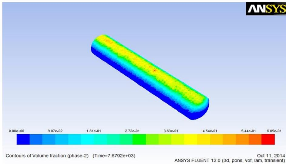
Figure 5. Methane allocation inside tank
