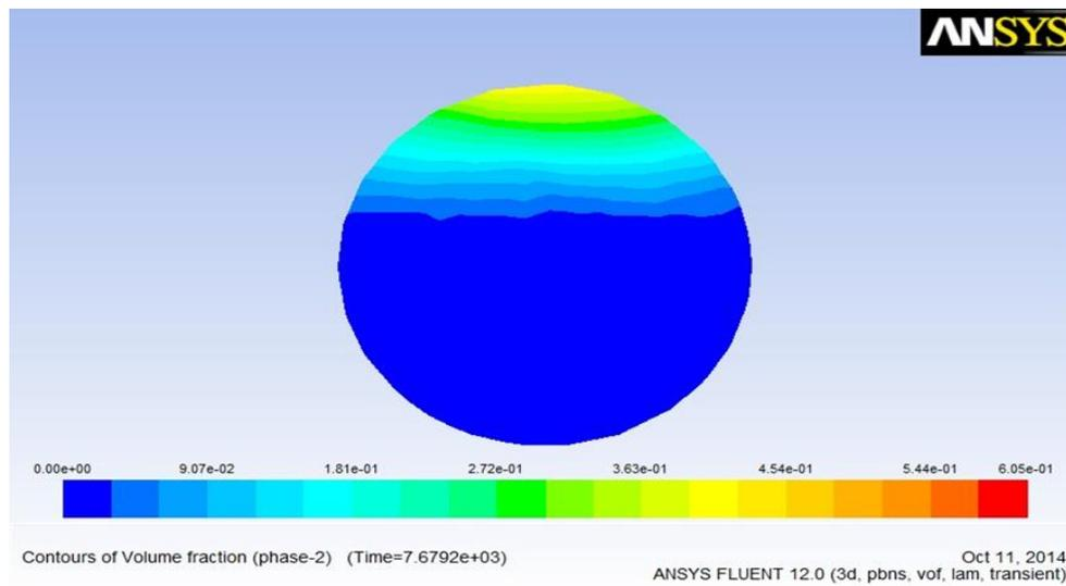
Figure 7. Methane allocation at z-axis symmetric plane
