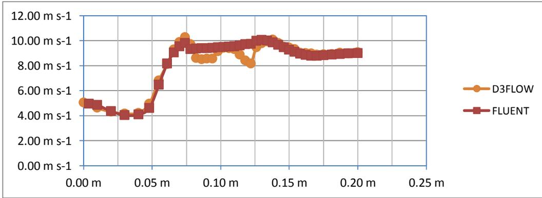
Figure 12. Velocity magnitude (m/s) distribution comparing D3flow–Fluent results for upper–left side
