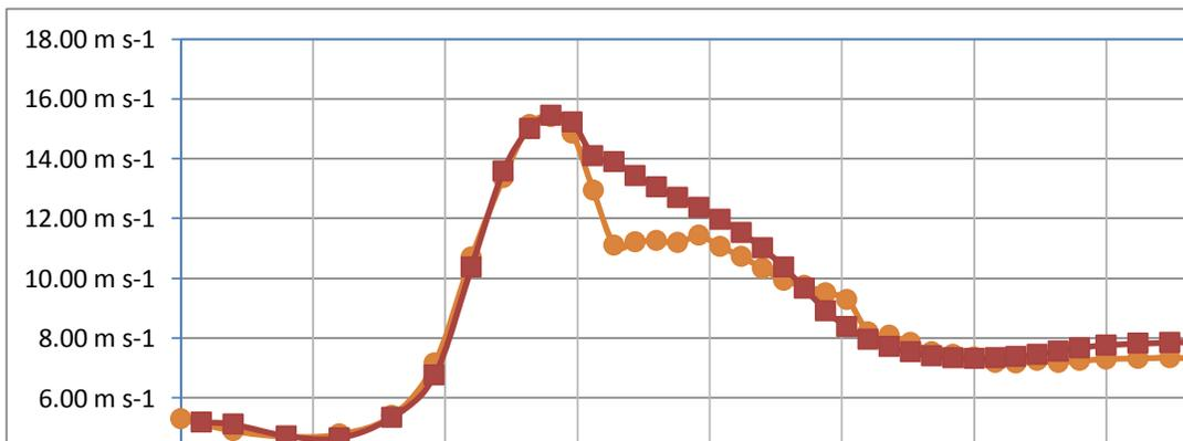
Figure 11. Velocity magnitude (m/s) distribution comparing D3flow–Fluent results for upper – right side
