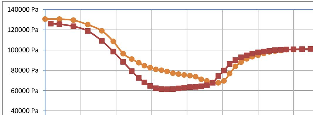
Figure 5. Static pressure (Pa) distribution comparing D3flow–Fluent results for bottom–right side
