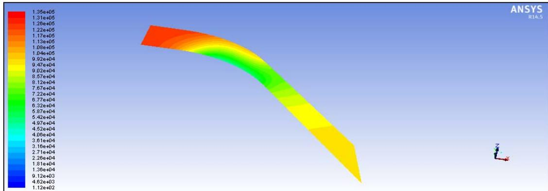
Figure 13. Contours of static pressure (Pa) at the bottom side using Fluent
