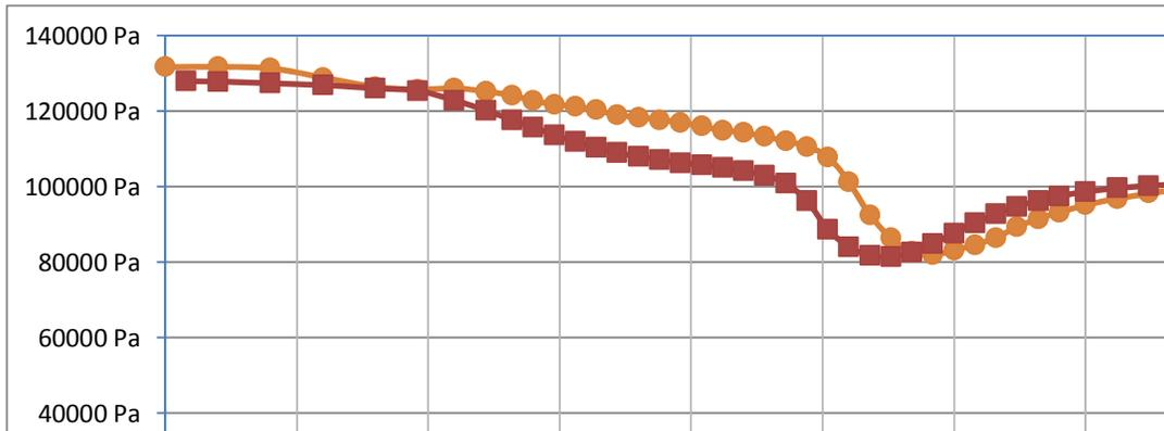
Figure 6. Static pressure (Pa) distribution comparing D3flow-Fluent results for bottom-left side
