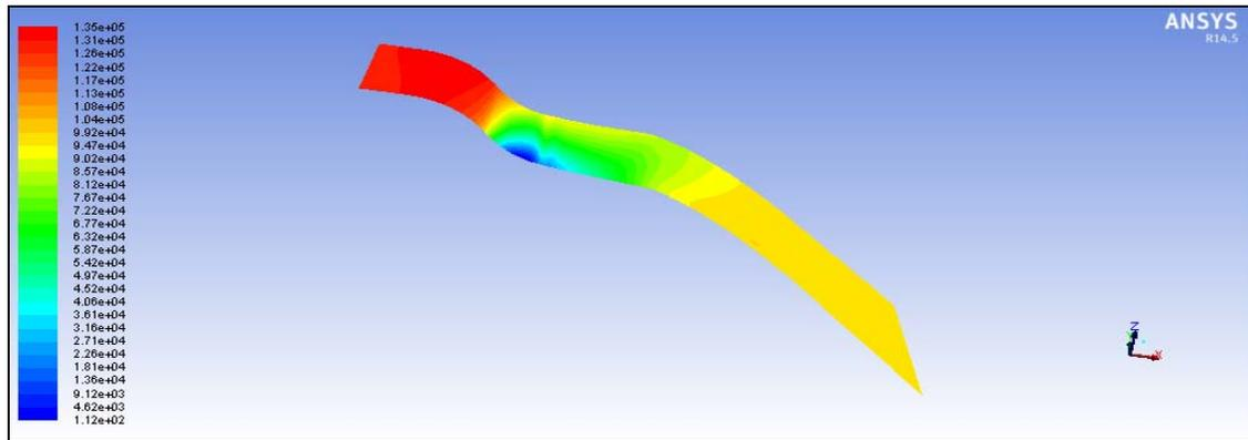
Figure 14. Contours of static pressure (Pa) at the upper side in Fluent
