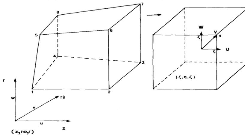
Figure 2. Distorted cubes of the physical domain are mapped into cubes of the computational domain
