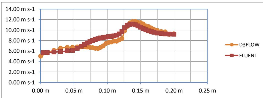
Figure 10. Velocity magnitude (m/s) distribution comparing D3flow–Fluent results for bottom–left side
