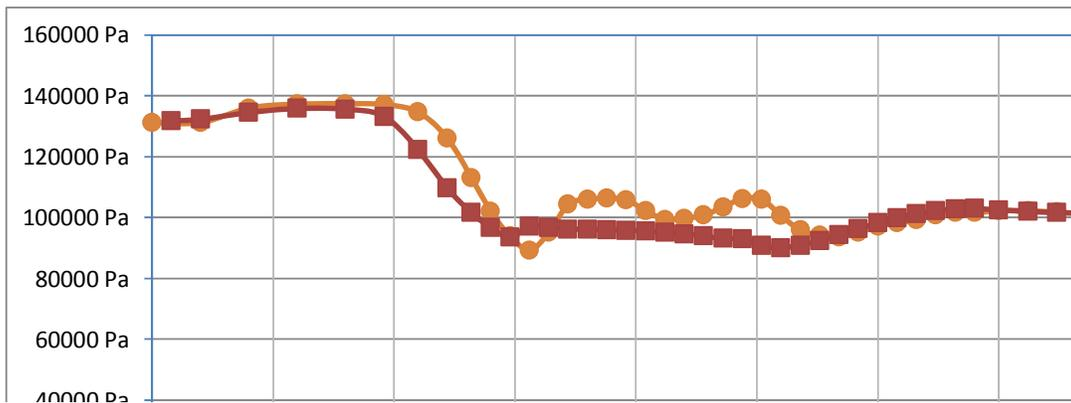
Figure 8. Static pressure (Pa) distribution comparing D3flow-Fluent results for upper-left side
