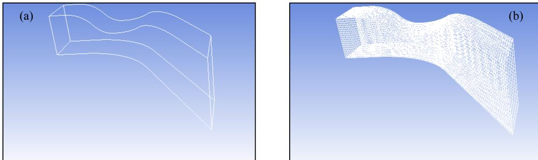
Figure 1. (a) Geometry of the 3D nozzle, (b) mesh used for analysis (Fluent)
